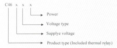
X: C-46 type solenoid valve coil are used with by valves.
