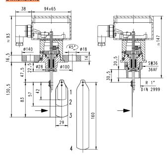
Adapt paddle 1 for DN 25. From DN 100, adapt paddle 4: DN 100 Paddle length 92 DN 125 Paddle length 117 DN 150 Paddle length 143 from DN 175 unshortened Attention! Flange seal not included in scope of delivery
