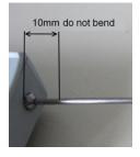
Do not bend at a point closer to the bolting than 10mm.
