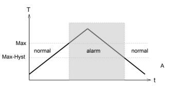
switchover delay time  $(t_{\text{DS}})$  can be applied to the switchover to the alarm state. Equally, one switch-back delay time  $(t_{\text{DR}})$  of several can be applied to switching back to the normal state.
