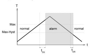
In the normal state the integrated LED is on, in the alarm state it is off, and this corresponds to its status when there is no supply voltaae.
