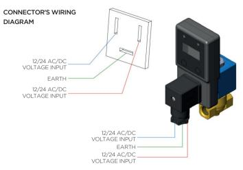
**Note:** The device is able to function properly at 12 and 24 volts together with AC or DC voltage. Through the rectifier circuit that is in the timer, the device is open to any connection apart from either there is a connection order between DC voltage with + and - cables or AC voltage with phase or neutral cables, or not.
