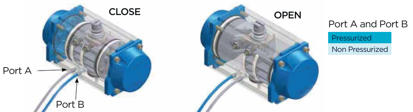
Fig 2. Double Acting Actuators
